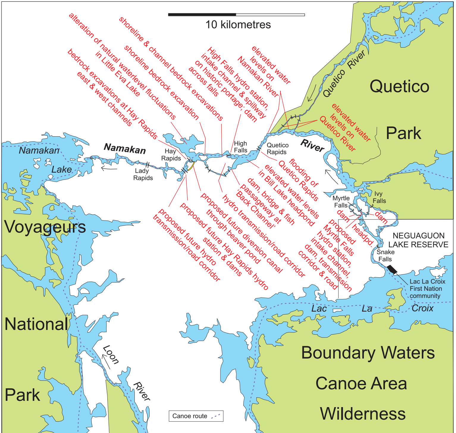
FIGURE 2: PROPOSED HYDRO-ELECTRIC DEVELOPMENT ON NAMAKAN RIVER
